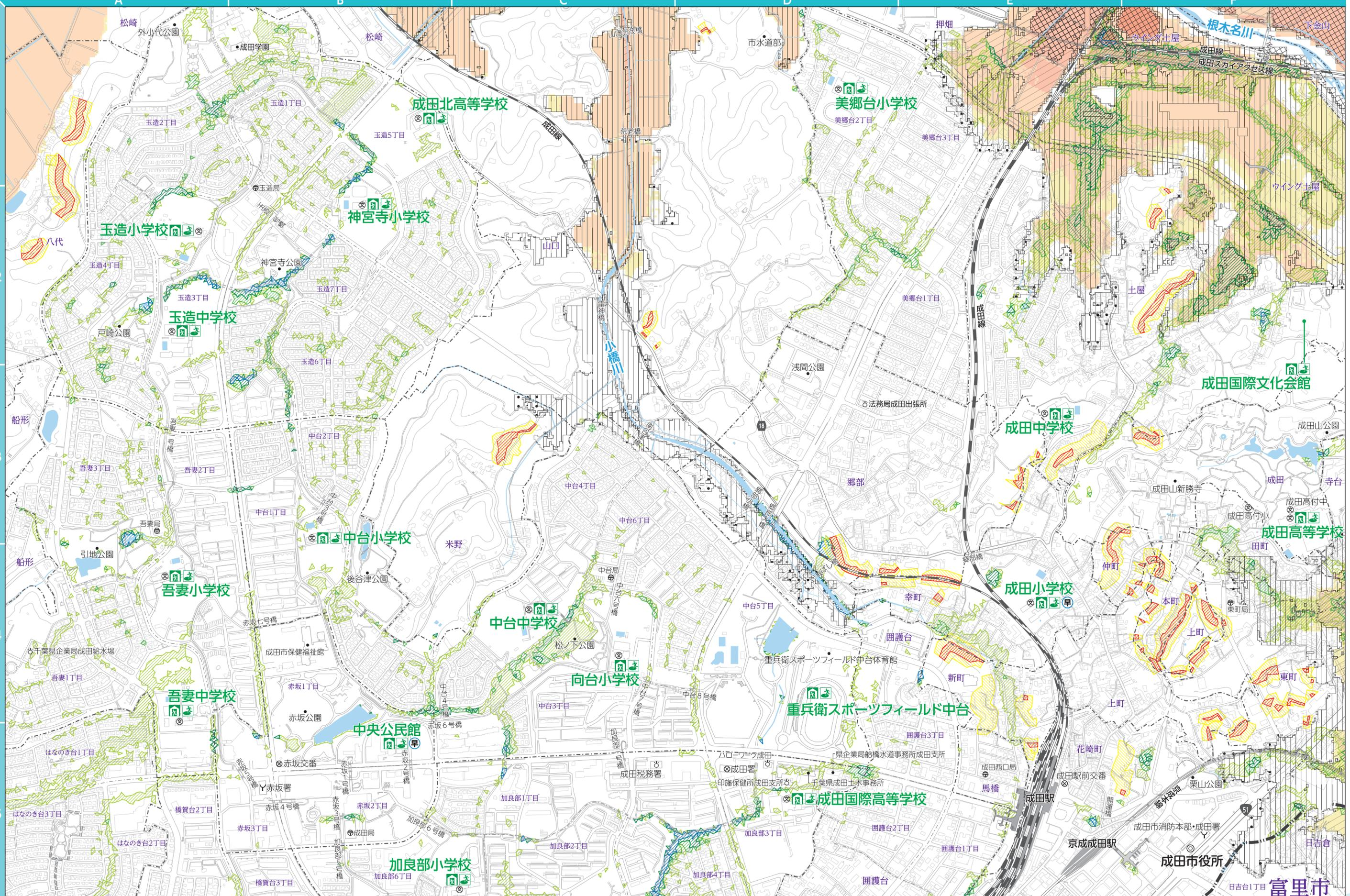
Legend Inland flood predicted area 0.05 m-less than 0.3 m 0.3 m-less than 0.5 m 0.5 m-less than 1.0 m 1.0 m-less than 3.0 m 3.0 m-less than 5.0 m
